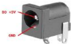
External DC Power supply port (J1), supply voltage from DC5V-9V. (Center positive)
