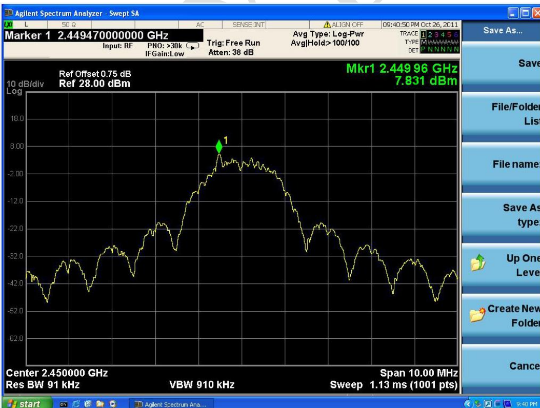
Figure 3-26. Modulating Signal Testing
